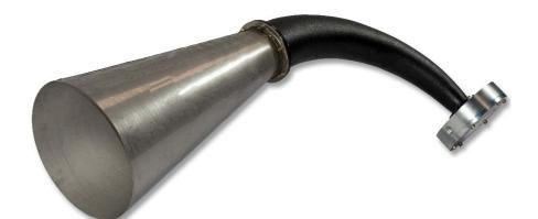
ACS acoustic cleaners use compressed air to flex a titanium diaphragm to produce pressure pulses that are amplified by the bell. The resulting low frequency/high energy sound waves that are emitted resonates/dislodges particulate deposits. The displaced particulate deposits are then removed by gravity and/or gas flow.
